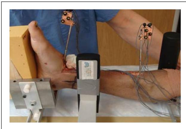
**Figure 1.** Telos ankle stress apparatus at neutral ankle dorsiflexion.
