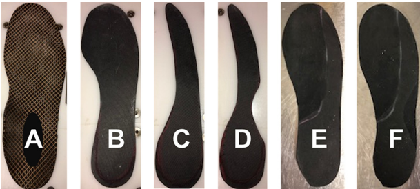
Figure 2. Orthotic components were combined to form 11 conditions, which were tested in a randomized order for each specimen. Images of components used in orthotic conditions include combinations of (A) a commercial orthotic device, (B) a full-length carbon fiber plate, (C) a full-length lateral carbon fiber plate, (D) a full-length lateral cut carbon fiber plate, (E) a full-length lateral foam wedge, and (F) a full-length lateral cut foam wedge.
