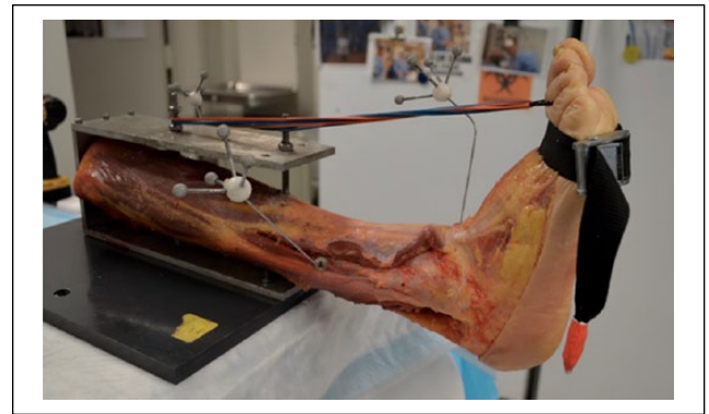
Figure 1. Experimental setup. The tibia is secured to the testing frame with 2 threaded rods. A canvas strap is attached to the forefoot for external rotation stresses, and the marker clusters for motion capture are rigidly secured to the bone with screws. The foot is held in neutral dorsiflexion position with elastic bands.
